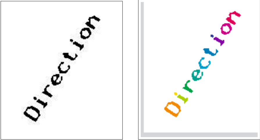
Fig. 17.5. (Left) A binary image with several regions. (Right) A connected component labelling where colors represent labels
